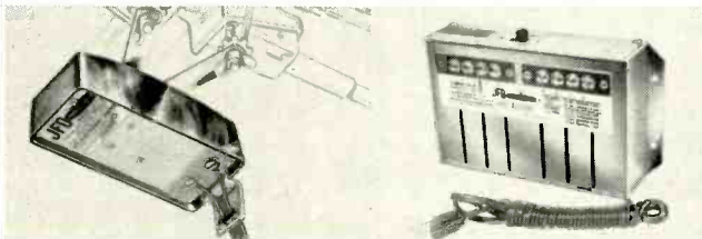
amplifier is mounted directly on antenna terminals
