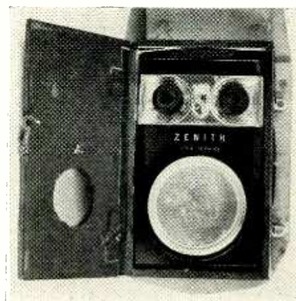
Receiver end of locator. Receiver box is open, showing transistor radio inside.
