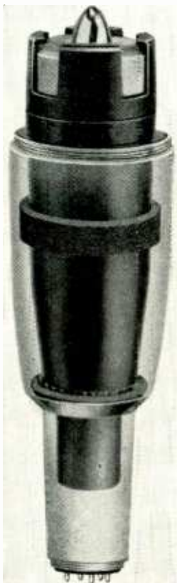
Phantom view of cardioid dynamic modular mike. Clear plastic shell is used here to show shock mounting on which the inner metal case floats.
