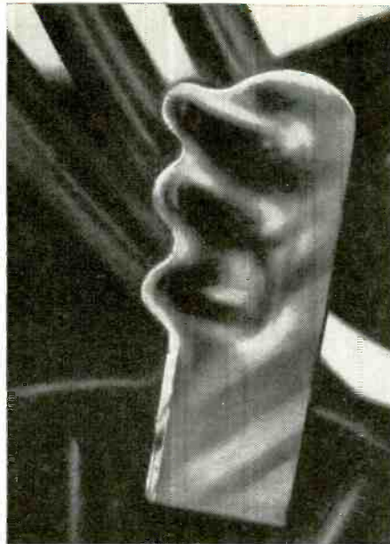
GOOD SOLDER JOINT • Good wraps • Joint well filleted • Outline of wires visible through solder
