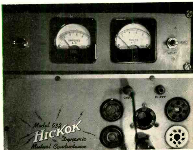
Fig. 1—0-1 ac ammeter added to tube tester. Unit is connected in series with the common heater transformer winding.
