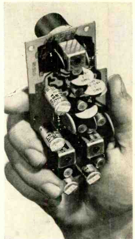
Transistorized remote control amplifier draws only 0.8 watt and can be left on standby indefinitely at negligible cost.
