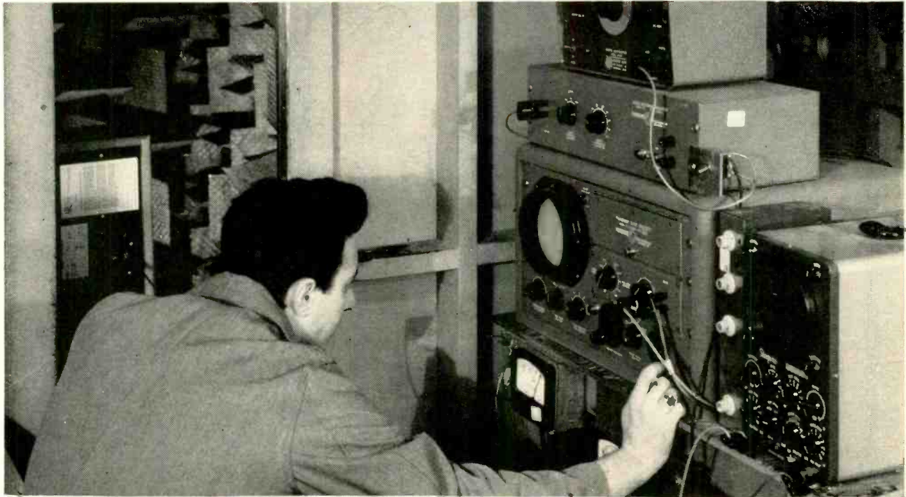
Silvano Cannavacciuolo, AR inspector, checks a speaker response curve at one of AR's anechoic chambers. The response curves of the individual drivers in the system he is testing have already been recorded and found acceptable at the main anechoic chamber.
