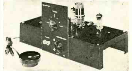
RADIO RECEIVER, Kit-tronics RB-10 , 3-stage, 2-tube, receives local broadcast stations. 1-tube regenerative receiver, 1-tube power amplifier and transformer-type half-wave power supply
