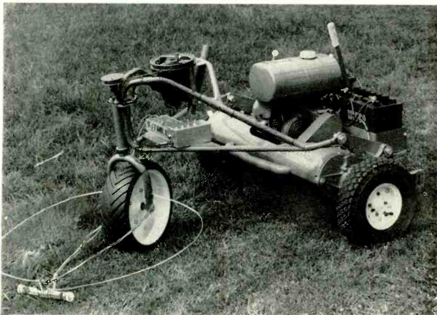
With all electronics mounted, the mower is ready to go. Hoop-like wire around front wheel is safety device.
