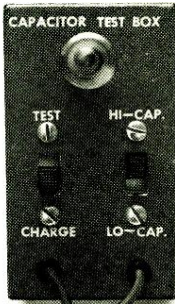
Completed electrolytic tester.
