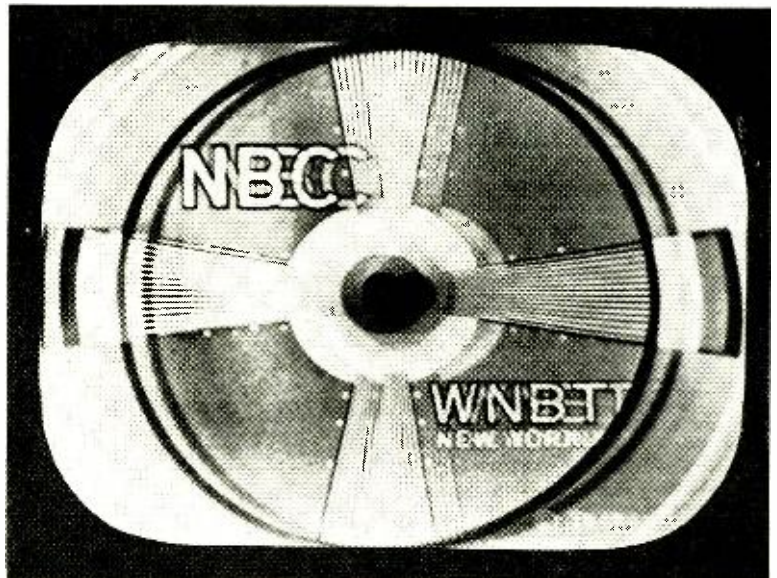
This trailing ghost was caused by a reflected signal.
