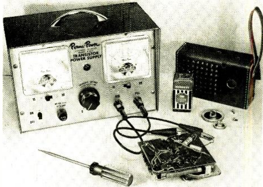
Bench setup for checking transistor radios. A continuously adjustable power supply is a great convenience.
