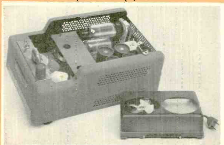
Under the hood, layout is simple. Note TV type horizontal output tubes which act as power amplifiers.
