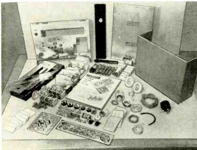
Spread out kit components for check against parts list before starting construction.
