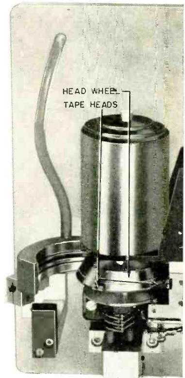
Fig. 1—Motor and head-wheel assembly with open vacuum shoe.
