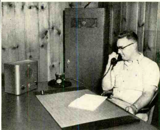
Transmitter, receiver and power supply at base station are in rack cabinet in corner. Control unit is on desk.
