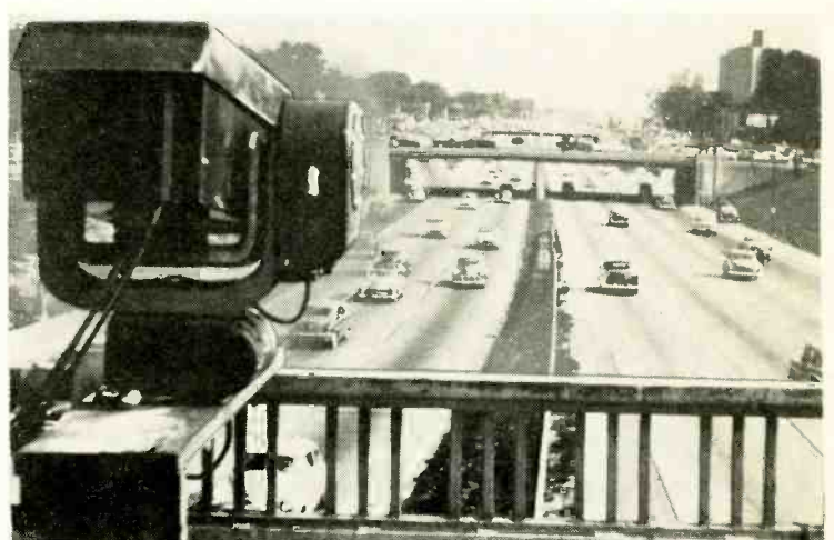
Closed-circuit TV scans a Detroit expressway in recent test. A more extensive experiment is planned, using 33 cameras to patrol an eight-mile stretch. Roadside warning and detour signs will be activated from a central control room.
