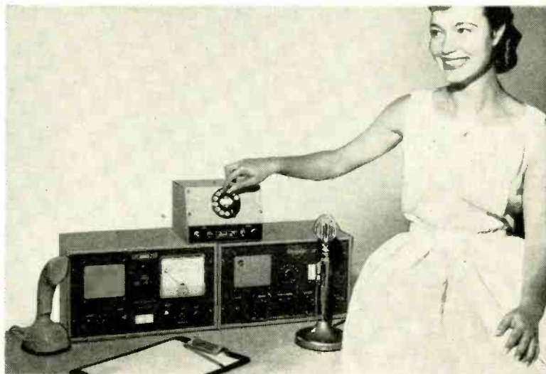
A remote-control point for a base station equipped with a dial type selective calling.
