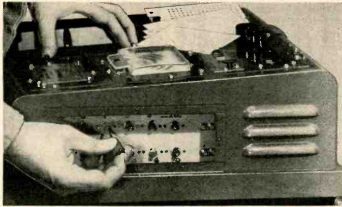
Fig. 4—Potentiometer adjustments are used in calibrating the instrument.
