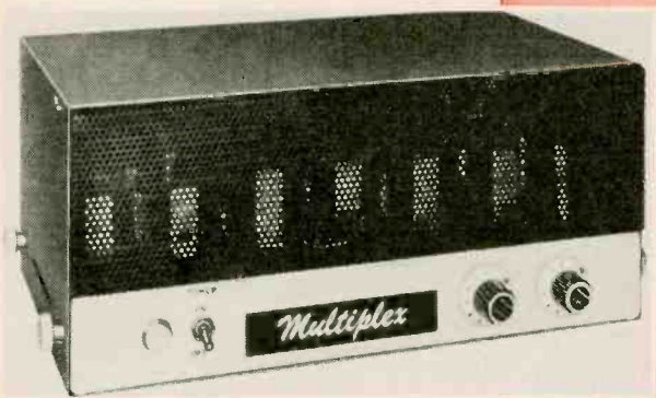
Bogen model RM-2, a crystal-controlled multiplex receiver.
