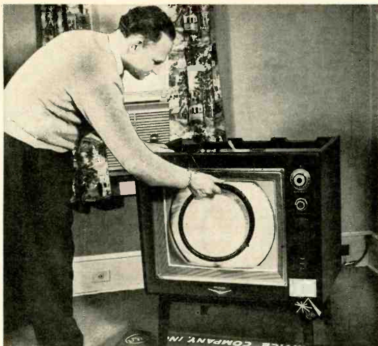
Using the degaussing coil on a color TV installation.
