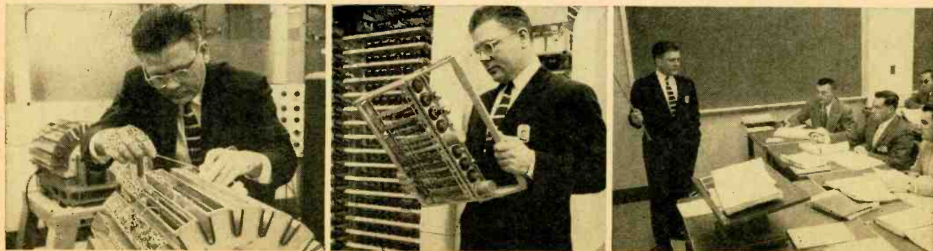
Brani trouble shooting Magnetic Drum Frame. Brani studies computer pluggable unit. Dick explains computer logic to a Systems Class.
