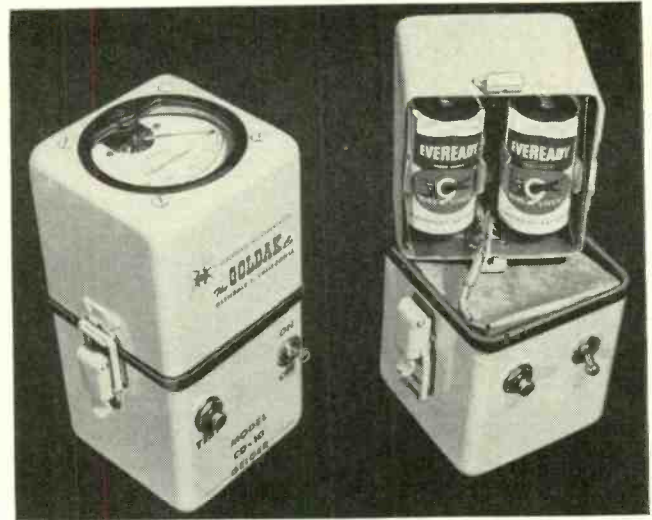
This Civil Defense radiation detector can be fastened to the wearer's belt.
