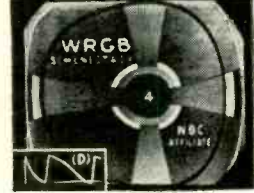
FAULT: Picture stretching at left and compression at right. CAUSE: 0.02 mf boost capacitor (connected to linearity coil) used instead of 0.1 mf capacitor. (D): H. Yoke current wave-form.
