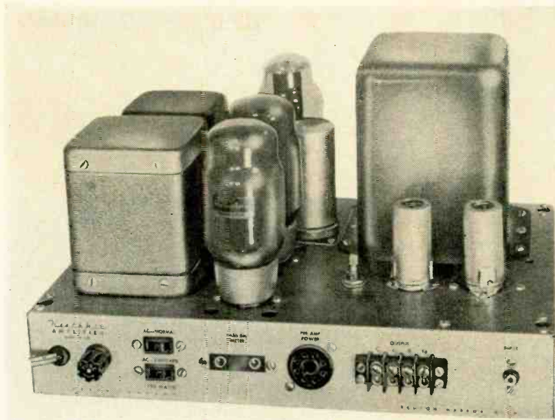
Amplifier without its cover. Output transformer is at left—power at rear right.
