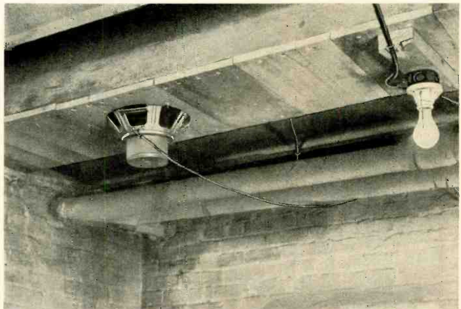
The Flewelling air coupler from below. From above it looks like a hot-air register.
