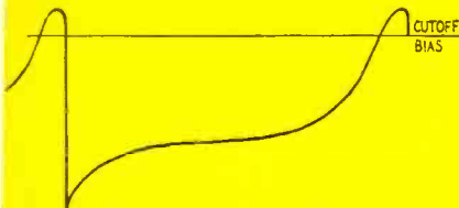
Fig. 3—Ideal grid-voltage waveform.
