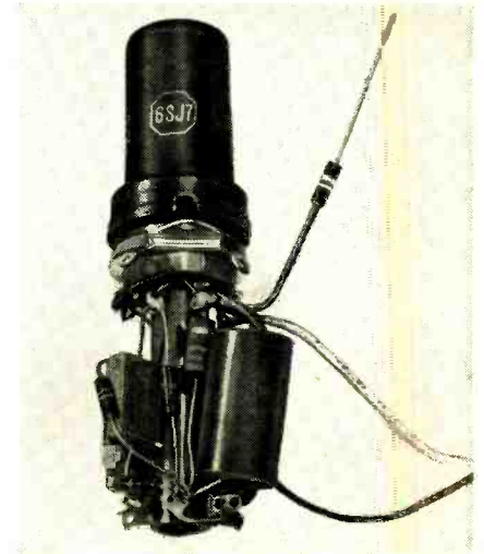
Phase-shift oscillator uses one tube.
