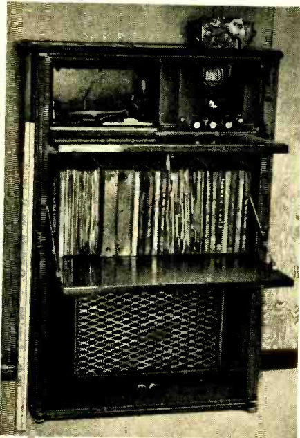
Photo of a combination cabinet with the 12-inch R-J type speaker enclosure.
