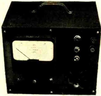
The relative field-strength meter simplifies antenna installations.
