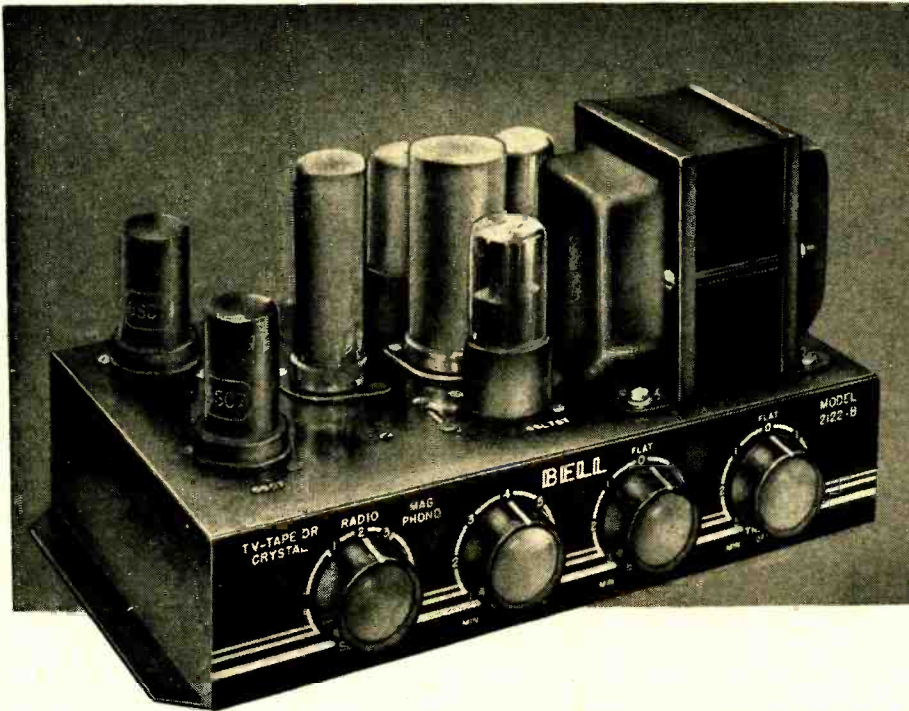
Typical high-quality audio amplifier—includes a phono pre-amp.
