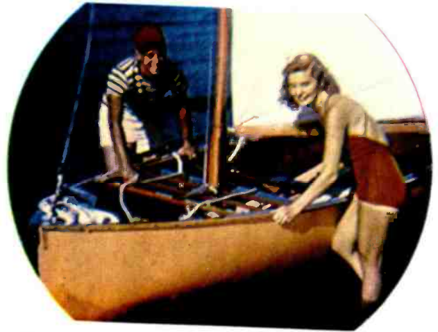
Fig. 13—Failure of "Q" signal produces reddish picture.
