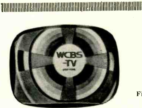
Fig. 3—Picture is improperly centered.
