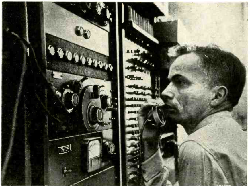
"AUDREY"—Bell Laboratories' Automatic Digit Recognizer—selects the right circuits automatically when numbers are spoken distinctly into the telephone.
