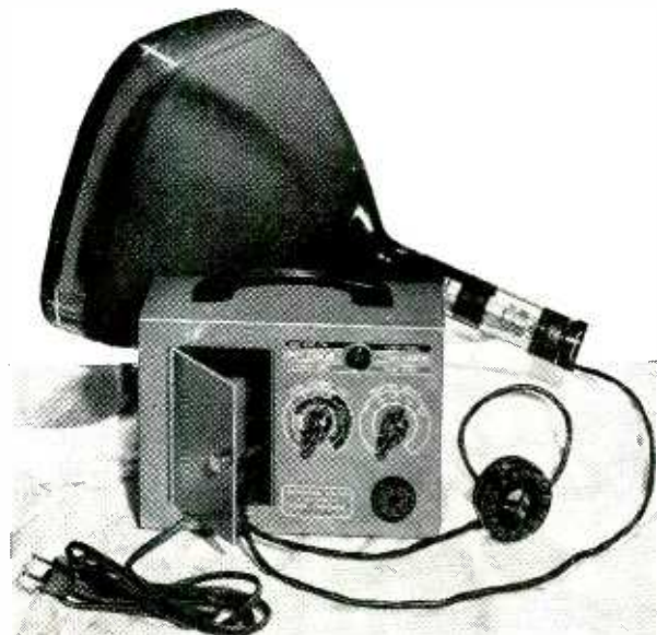
Fig. 6—National Union Videotron picture tube checker locates internal defects and shows useful light output.
