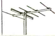
JC — The original and most popular five element Yagi.
