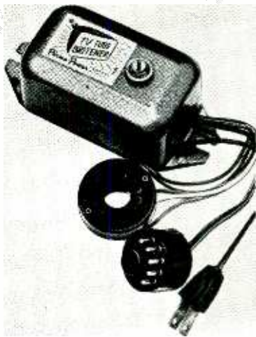
Fig. 10—Perma-Power "Britener" reactivates cathode by raising heater voltage.
