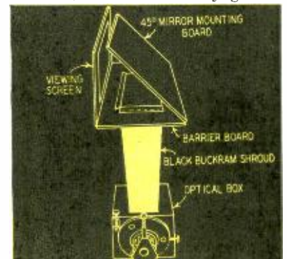
Fig. 3—The optical system is shielded from stray light and dust by a shroud.
