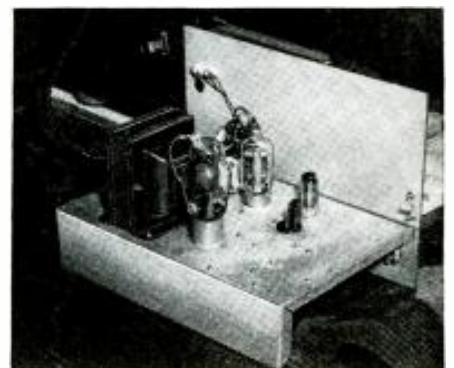
Rear view. Bias batteries are under chassis.
