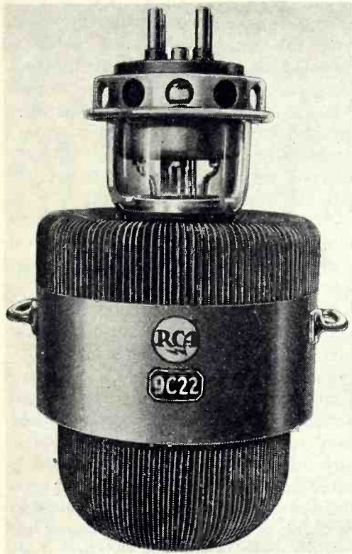
Fig. 1. An air-cooled transmitting triode showing the silver-soldered ventilating fins.
