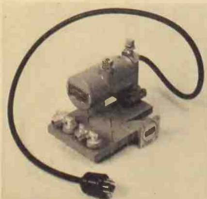
Double balanced mixer with local oscillator mount and variable attenuator.
