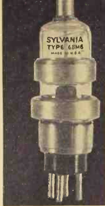
The Type 6BM6 reflex klystron uses only one toroidal cavity.
