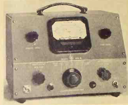
Hewlett-Packard Model 430 B microwave power meter for measurements to 3000 mc., depending on bolometer mount.
