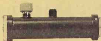
Miniaturized S-band cavity having a tuning range of 200 mc. or more at about 3000 mc.
