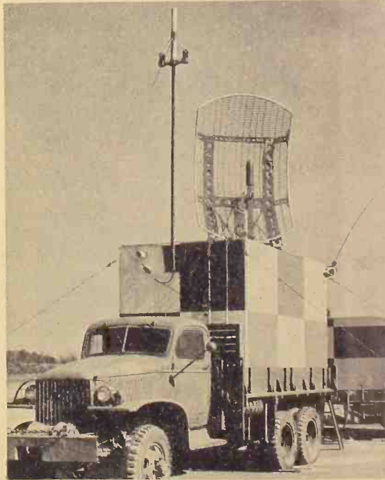
Fig. 7. Airport surveillance radar equipment mounted in truck and trailer.
