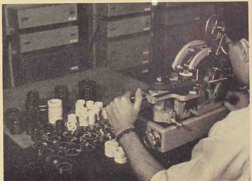
Toroidal coil winding operation at the plant of Lenkurt Electric Co., Inc.
