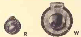
MODELS R AND W DUODIALS Each model available in standard turns-ratios of 10, 15, 25 and 40 to 1. Inner scale indicates angular position of HELIPOT sliding contact, and outer scale the helical turn on which it is located. Can be driven from knob or shaft end. R—2" diameter, exclusive of index. W—4-3/4" diameter, exclusive of index. Features finger hole in knob to speed rotation.
