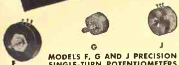
MODELS F, G AND J PRECISION SINGLE-TURN POTENTIOMETERS Feature both continuous and limited mechanical rotation, with maximum effective electrical rotation. Versatility of designs permit a wide variety of special features. F—3-5/16" dia., 5 watts, electrical rotation 359°—resistances 10 to 100,000 ohms. G—1-5/16" dia., 2 watts, electrical rotation 356°—resistances 5 to 20,000 ohms. J—2" dia., 5 watts, electrical rotation 357°—resistances 50 to 50,000 ohms.
