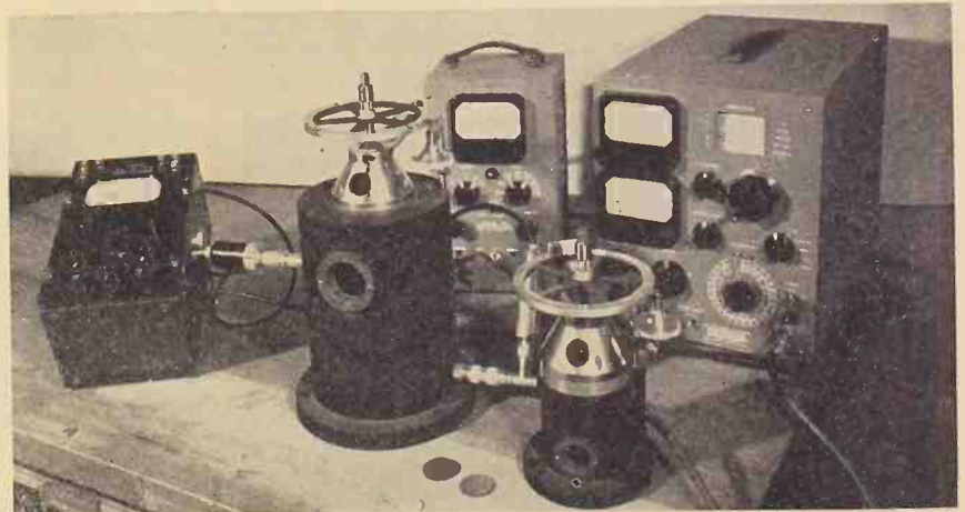
Resonant cavity apparatus for determining dielectric constant and power factor.
