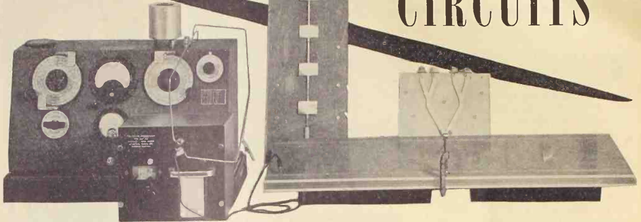
Setup for measuring the capacity of various transmission systems.
