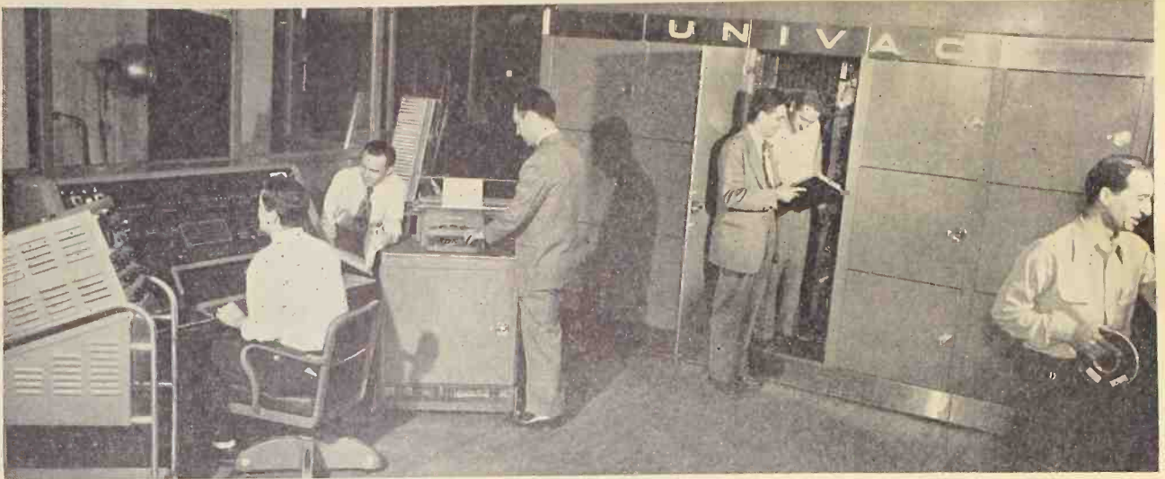
General view of Univac (Remington Rand) with central door open, partly revealing the "mercury memory" assembly.
