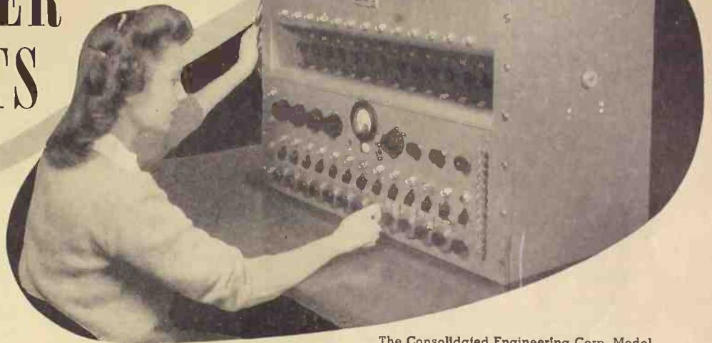
The Consolidated Engineering Corp. Model 30-103 electrical computer for solving up to 12 simultaneous linear equations.
