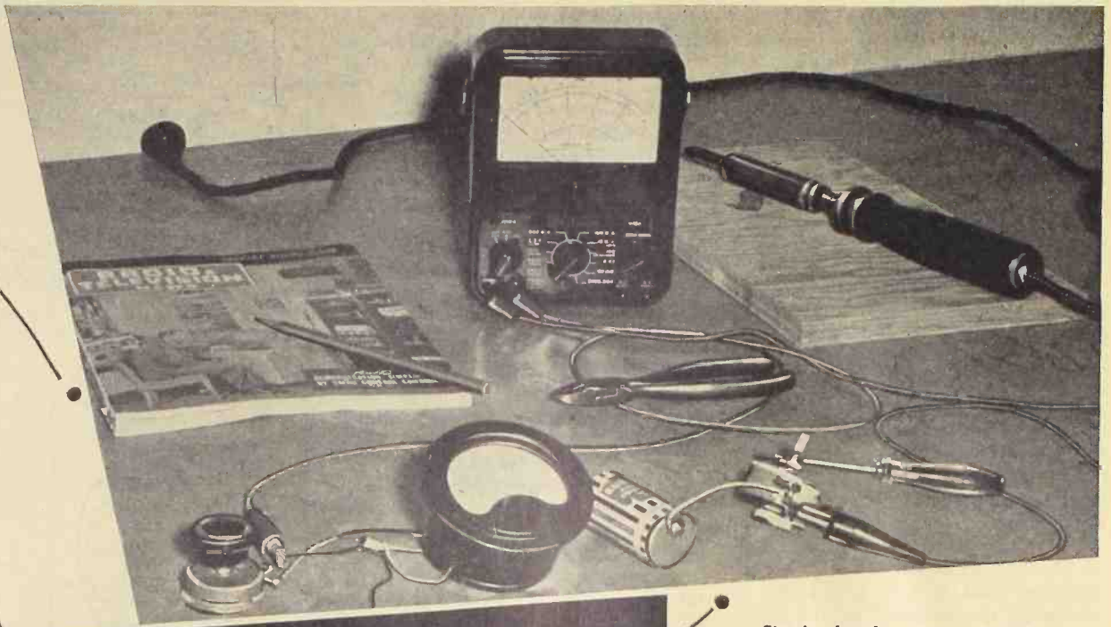
Simple bench setup required to run calibration curve on a.v.c. meter. Typical curve is shown in Fig. 2.
