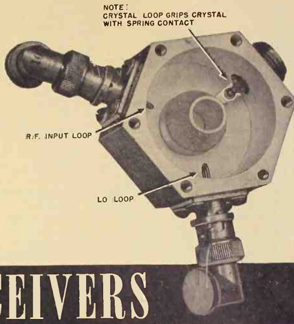
Fig. 2. Interior view showing r.f. local oscillator and crystal loops. The mixer employs a reentrant cavity and micrometer type tuning control.
