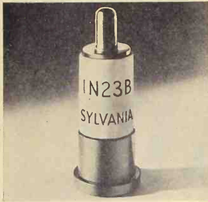
Fig. 10. Typical crystal designed for microwave mixers for use at frequencies in the 10,000 megacycle range.
