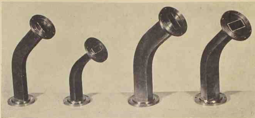
Fig. 11. Typical forty-five degree wave guide sections.
