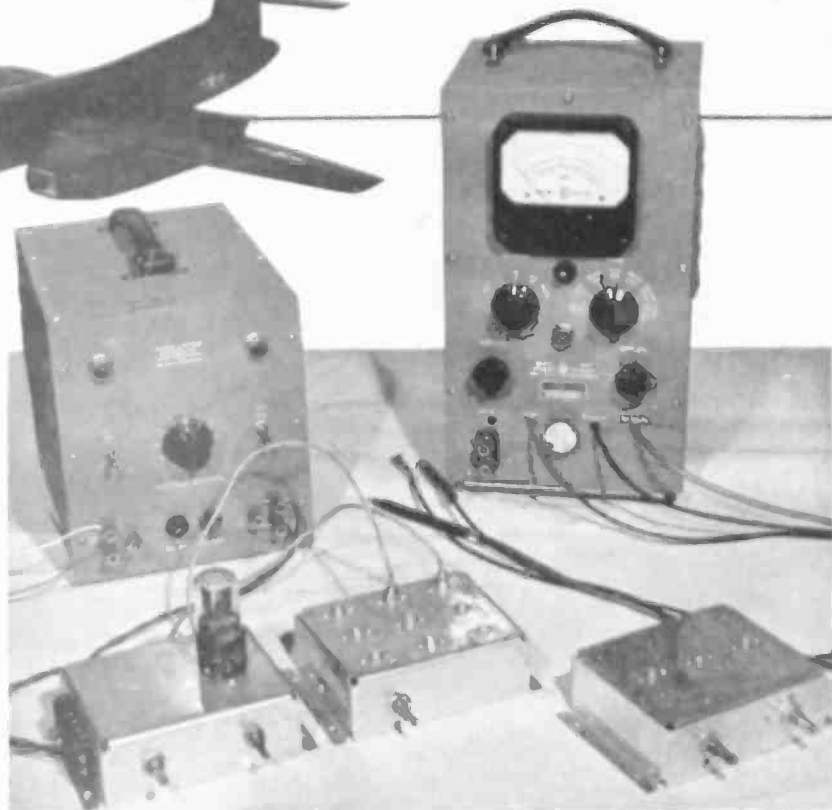
Fig. 1. D.c. amplifiers, a simple power supply, and some capacitive networks form a small electronic computer. Raggazini 6 has shown that such devices can simulate flight conditions of a new type airplane long before the first model is built. The aircraft shown is a Curtiss XF-8T.
