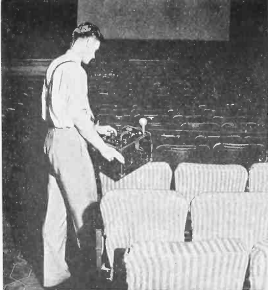
The General Radio type 759-B sound level meter being used to perform acoustic measurements in a motion picture theater.
