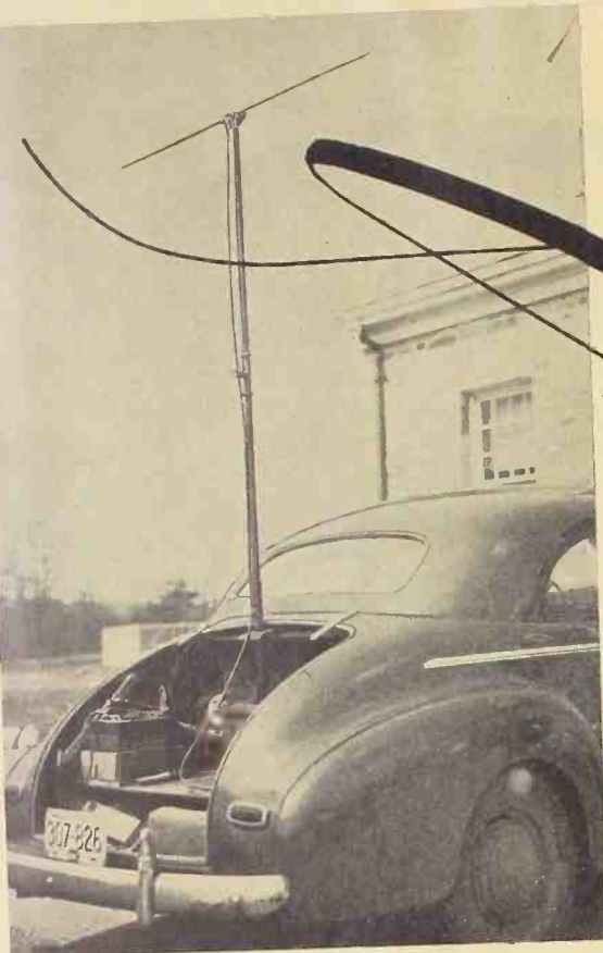
Rear view of car with trunk cover removed, showing how the antenna is mounted.
