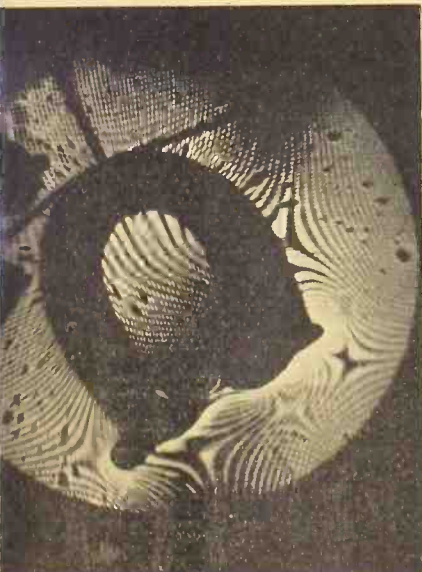
The magnetic field about a small horseshoe magnet, photographed by means of the new electron-optical shadow technique. Here the screen of an electron microscope shows the electron shadow of a fine wire mesh distorted by the deflection of the electrons as they pass through the field of the magnet. Total width of the magnet is about one-fourth inch.
