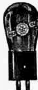
Type 68X-218B For use in battery aligning circuit to rectify alternating current — advantageous in supplying the higher cur- rent required by power tube equipped sets. List price $7.50
