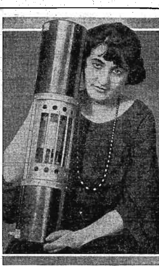
The largest and most powerful English vacuum tube was placed on exhibition in this country recently. The tube, held by Mrs. H. Lesser, is a five-kilowatt tube, and was sent to the Radio department of the navy for test and research work. The tube is valued at $1,500 and was brought to the United States by special messenger.
