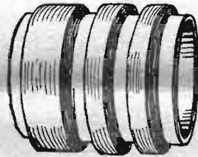
Figure 19—Bank-wound coil divided into sections
