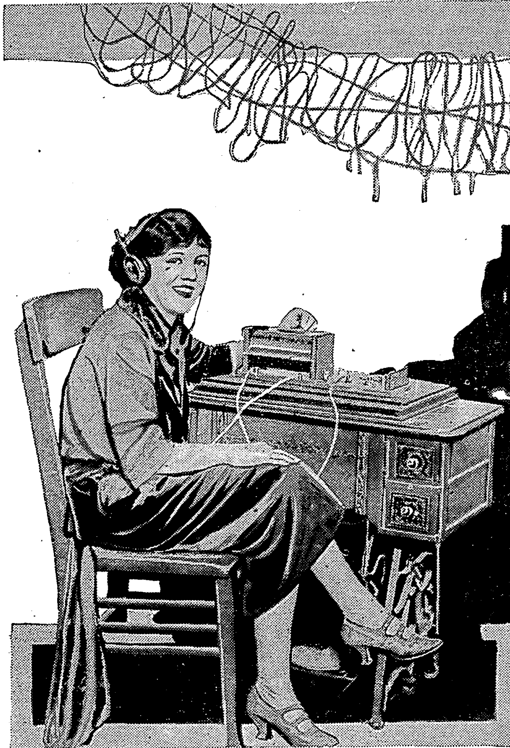
Miss Mabel Goodman, girl Radiophan of New York City, has found a new use for mother's sewing machine, as this picture testifies. Miss Goodman built the receiving set and cage-type aerial herself and erected it. Results, she declares, are very satisfactory © K. & H.
