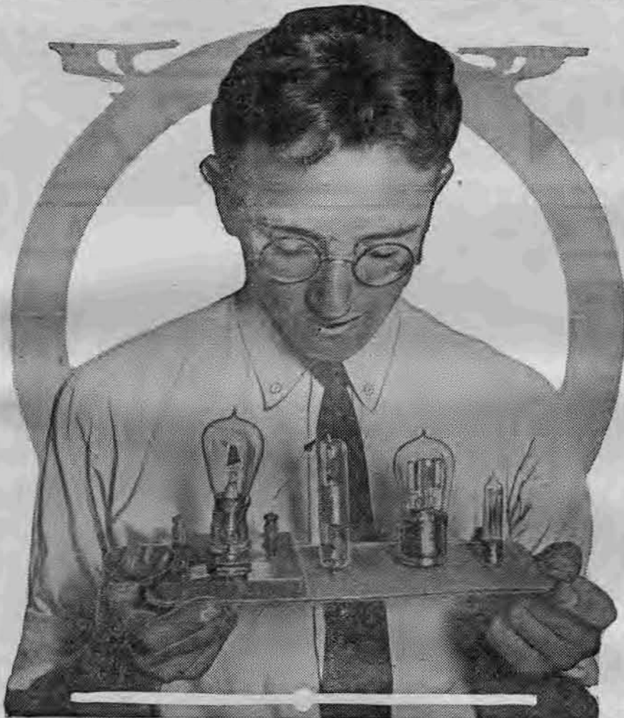
Rather than larger, vacuum tubes for Radio reception grow smaller with development. Starting at left, first is original two element tube of Dr. J. A. Fleming; second, later type with third element, the grid, added by Dr. Lee De Forest; third, is a modern type tube; fourth, "peanut tube," still in process of refinement. A. Ringel, City College, New York, is showing tubes.
