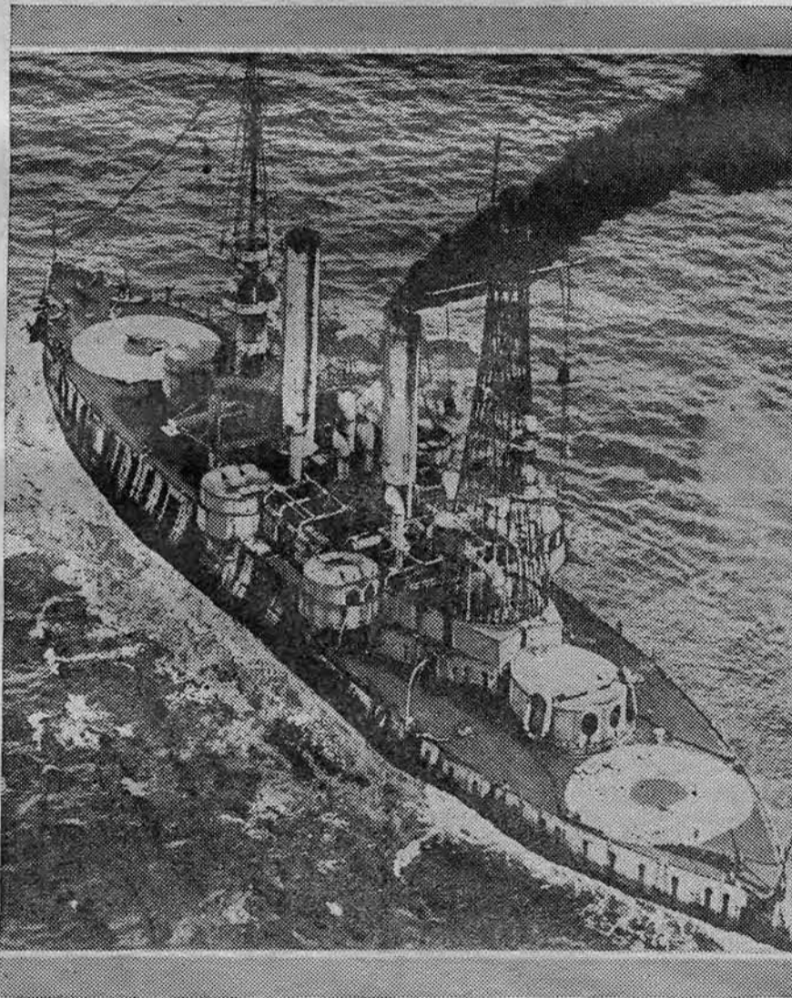
Here is the Battleship Iowa—not a man on board—doing all sorts of tricks off Virginia Capes in response to Radio signals sent from the Battleship Ohio, five miles away. The many successful tests of this new control device lead to a prophesy of manless wars.
