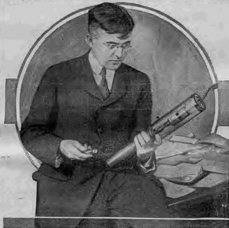
Dr. Langmuir compares 20 kilowatt and "peanut" tubes. Note end of plate protruding from large tube. This end is water-cooled
