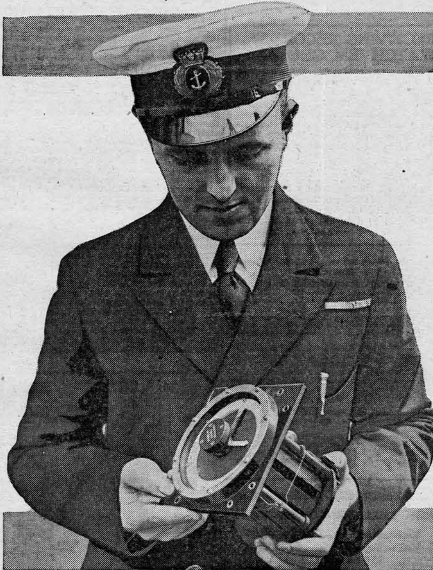
E. Brent, third Radio operator of the Majestic, holding the Gonia-meter from Marconi direction finder © Galloway, N. Y.
