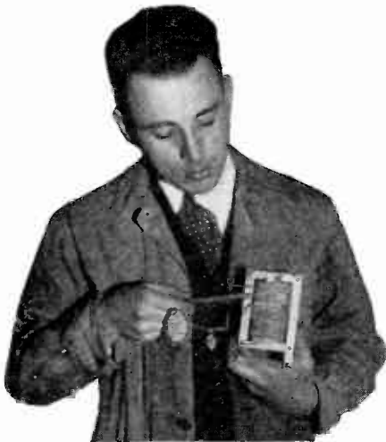
Mr. Ghirardi points out the windings on a typical "B" power transformer.
