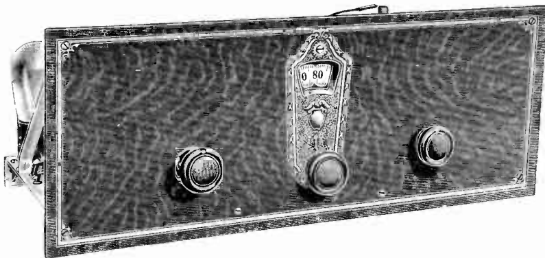
Front panel view of the K-121 model of the Country Special. This set will fit any 7 x 18-inch cabinet.
