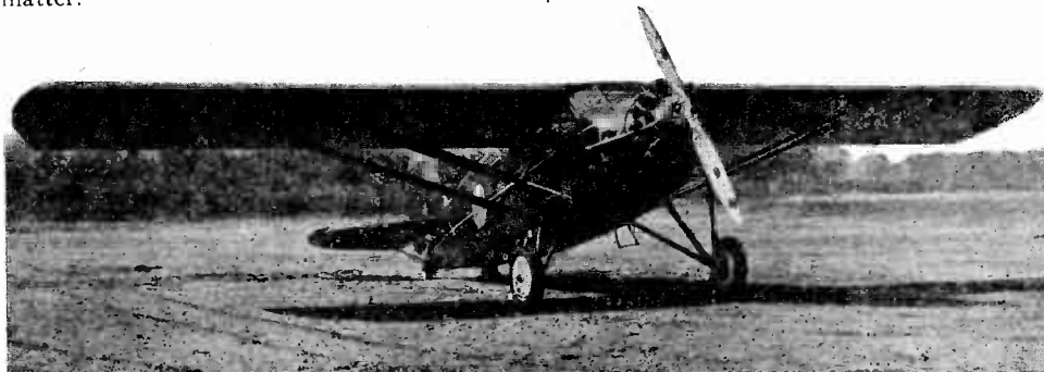
A view of the new monoplane just purchased by the Pilot Radio and Tube Corporation for use as a flying laboratory in the development of radio altimeter and other aircraft radio equipment. This plane, powered with a 300 h.p. engine, replaces the other ship described and pictured in past numbers of "Radio Design."
