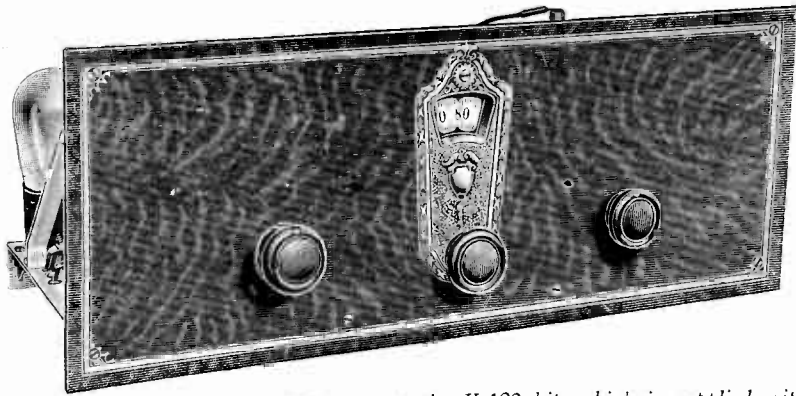
Front view of a P.E.6 assembled from the K-122 kit, which is supplied with a separate front panel. This model may be mounted in any standard 7 by 18 cabinet or console.
