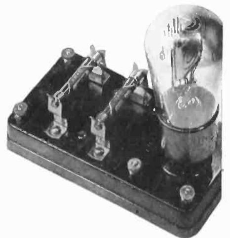
Above: All battery tubes and the 226 A. C. tubes can be used in the resistance coupler Redi-Blox. A 171 or 210 can be put in the last stage, and run with 5 volts A. C. on the filament. The rear resistor is in the plate circuit, while the forward resistor is the grid leak. Standard resistance values should be used. A very fine amplifier can be made with two transformer Redi-Blox and a resistance Redi-Blox between them. In such an outfit, both resistors should be of 2 megohms.
