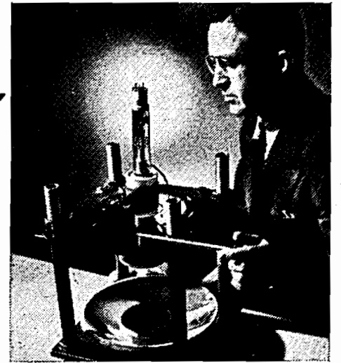
Dr. D. W. Epstein with a projection television tube, reflector and lens unit. Here the image on the end of the tube hits the reflector, is corrected by the lens, projected to the screen, then enlarged . . . making possible larger and clearer television than ever before.
