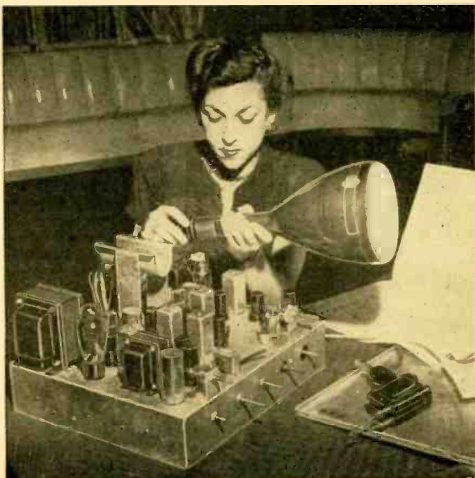
Partial prefabrication makes assembly problems much easier.
