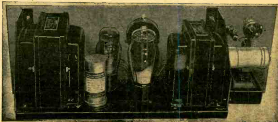
The power supply has a separate rectifier for the bias voltages.
