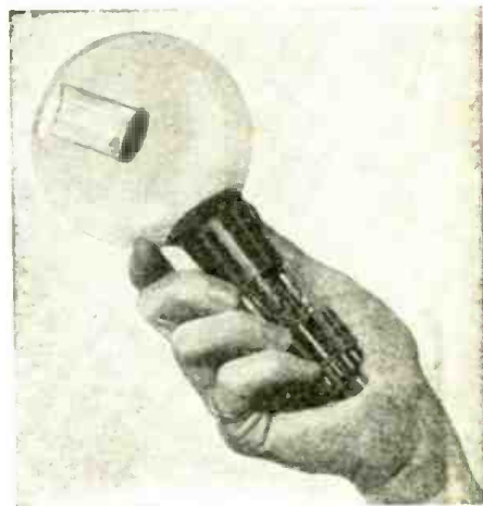
The special cathode-ray transmitting tube.
