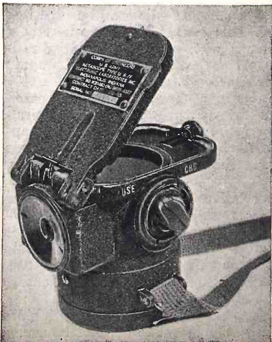
The Metascope, detector of infra-red light.
