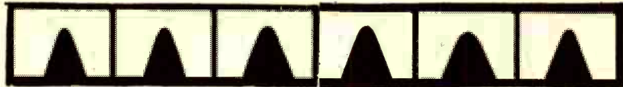
The various forms into which different types of needles wear, as seen in micro-photographs.
