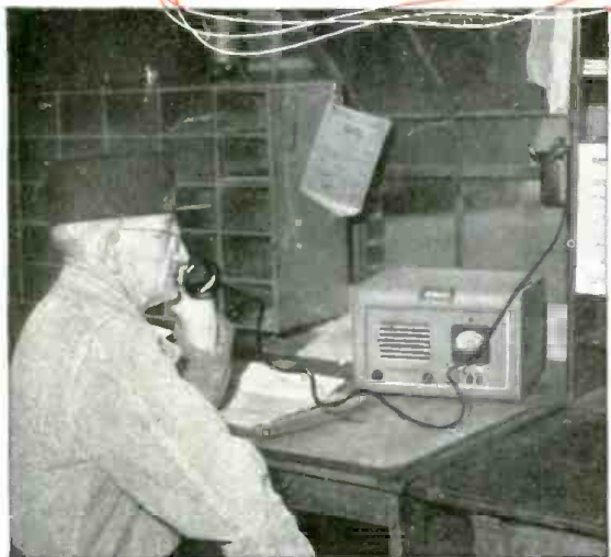
Photo shows yardmaster in Blue Island Yards of Rock Island Lines using his F-M two-way Motorola Radiotelephone to talk to freight engineer in his moving Diesel locomotive twenty-five miles away.
