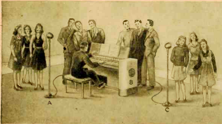
Altos are grouped around speaker A; basses near B; sopranos at C and tenors around the speaker in end of organ opposite B. Therefore each group is helped to sing in its own key.
