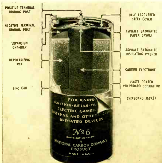
Fig. 4—Cut-away view of the dry cell whose internal workings are illustrated in Fig. 2. Construction details differ slightly in different makes of batteries, especially the smaller flashlight types and European cells.
