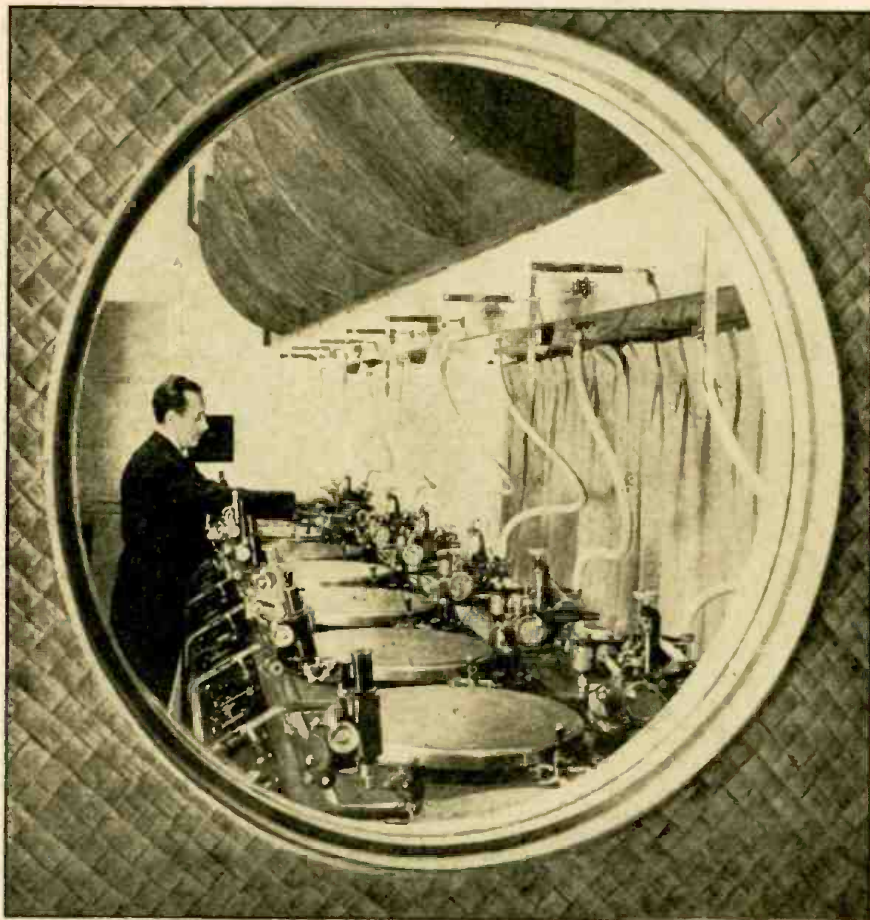
The battery of recording machines in the reference recording room of WOR's recording studios. Note the microscopes for examining the grooves, and the hoses of the exhaust system which takes away the minute chips and cuttings. Fourteen channels are available at all times, for "off-the-line" or "off-the-air" recording.
