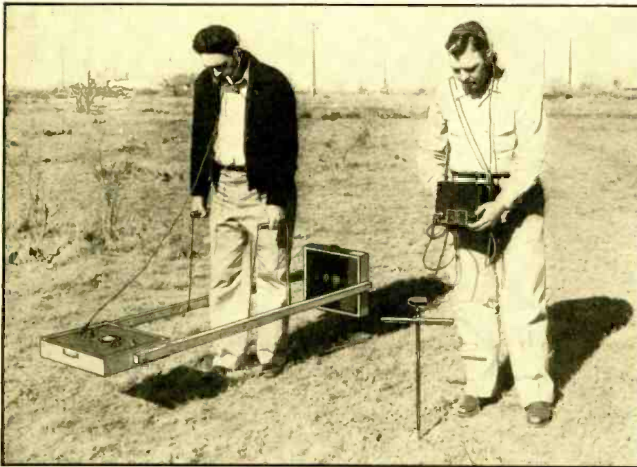
The completed Leak Detector (right) is used only after the Metal Locator has traced the underground path of the pipe. The latter is here shown during the process of completing this important initial step. The second and final step, next to repairing the actual leak, is to probe through the ground, until contact is made with the pipe, at 50-foot distances until the sound of the leak is heard. The vibration pickup (crystal microphone) is on top of the probe.
